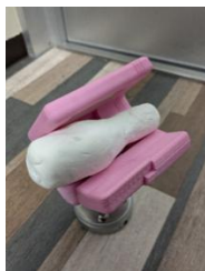
Figure 6 Creating a robotic hand for transporting chicken wings
