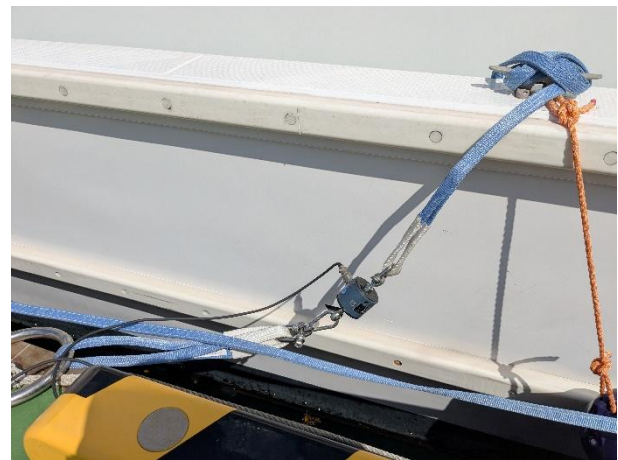
Figure 3. A tension load cell (LTM-1KN) attached to a mooring line.
