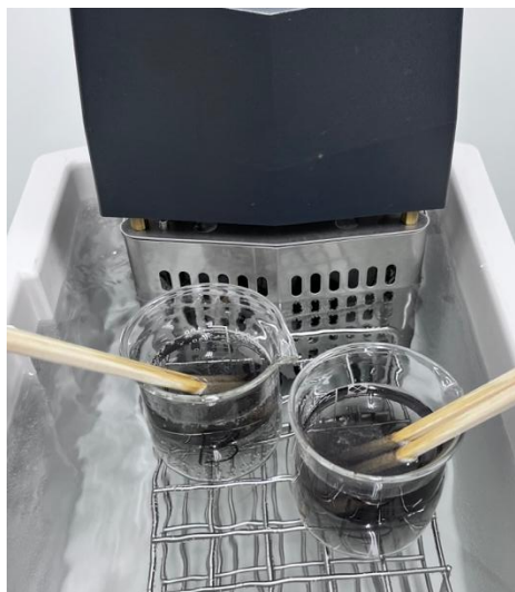
Figure 6: Enkianthus perulatus leaves undergoing electroless nickel plating.
