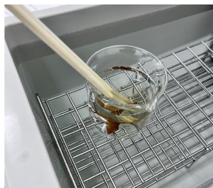
Figure 5: Applying a copper catalyst to Enkianthus perulatus leaves.
